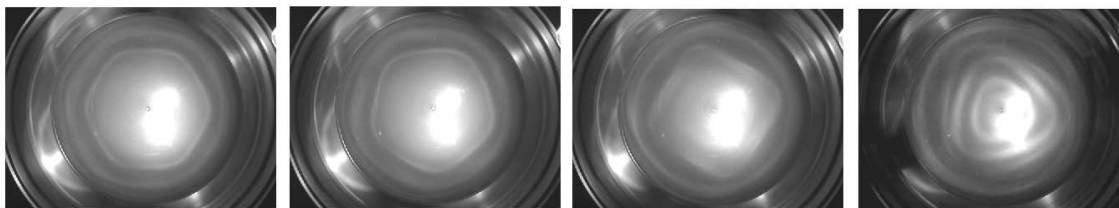
Figure 4: Photographs of the experiment, showing m_0 = 6, 5, 4 and 3 modes, just as in Fig. 3.
