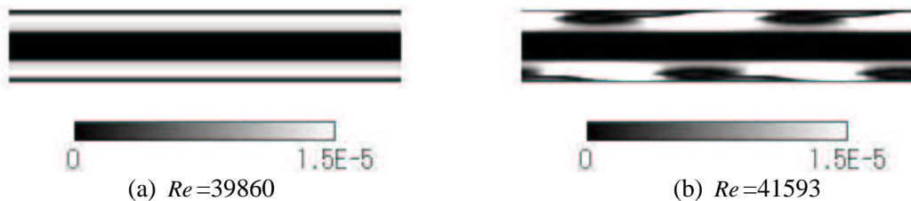
Fig.2 Variations of the axial velocity component in the \theta - z plane ( r_d = 0.954 , r = 0.412 ).
