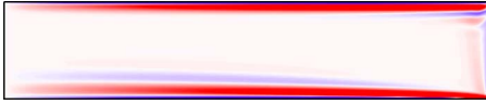
FIG. 2. (Color online) Contours of azimuthal vorticity \eta for the steady basic state at \text{Re}=5 \times 10^4 and \gamma=0.2 using n_r \times n_z=96 \times 48 and \delta t=5 \times 10^{-3} ; the contours are in the range \eta \in [-5, 5] .
