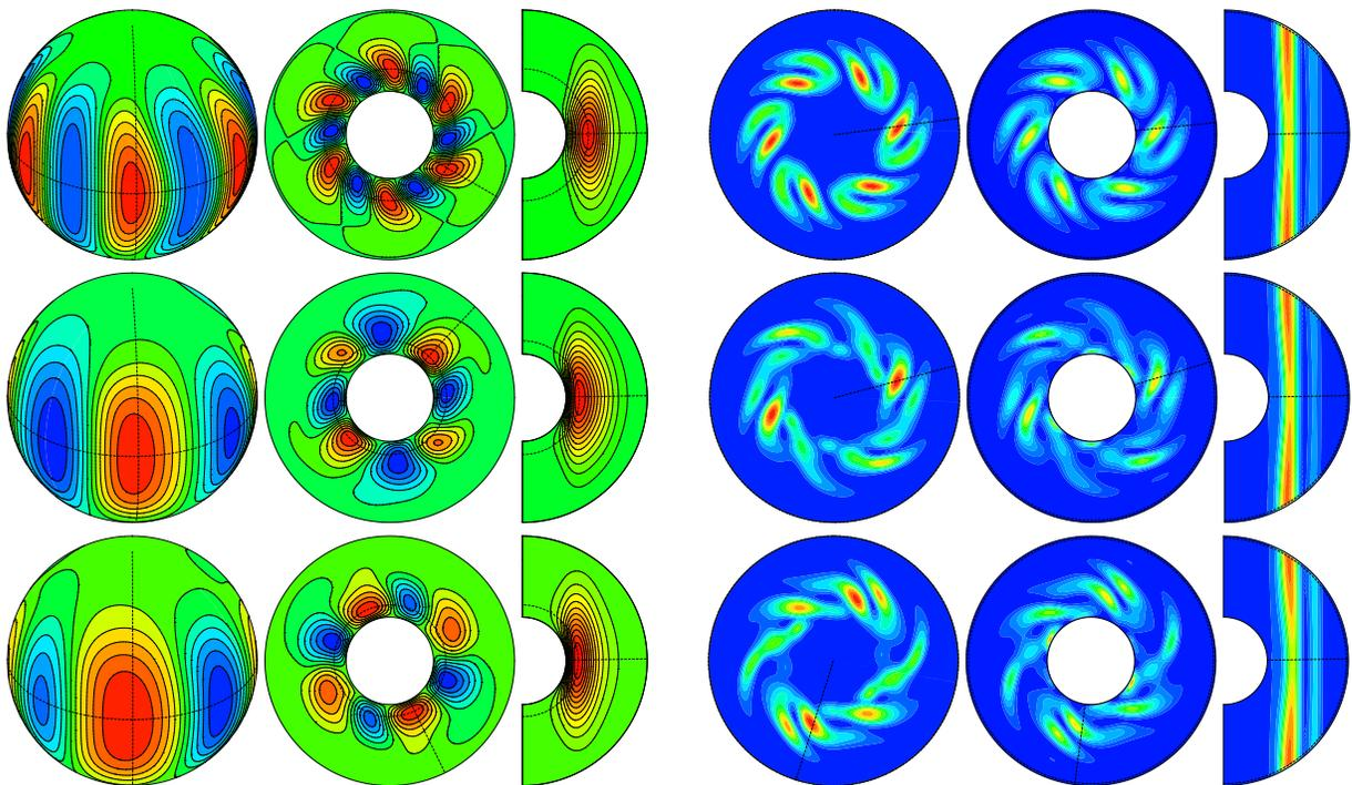
FIG. 10. Same contour plots as in Fig. 9 for the solution and the real and imaginary parts of the leading eigenfunction at the first Hopf bifurcation point ( $Ra_1^6 = 2.60701 \times 10^5$ ) on the six-fold branch.
