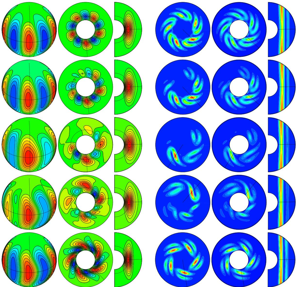
FIG. 6. The left column of three plots contains the contour plots of  $\Theta$  on a sphere, on the equatorial plane, and on a meridional section, for solutions lying on the  $m = 1$  branch of MRW at  $Ra = 2.04612 \times 10^5, 2.20259 \times 10^5, 3.23559 \times 10^5, 4.31323 \times 10^5, 4.87302 \times 10^5$  (from top to bottom). The right column corresponds to  $K$  for the solution and same  $Ra$ .
