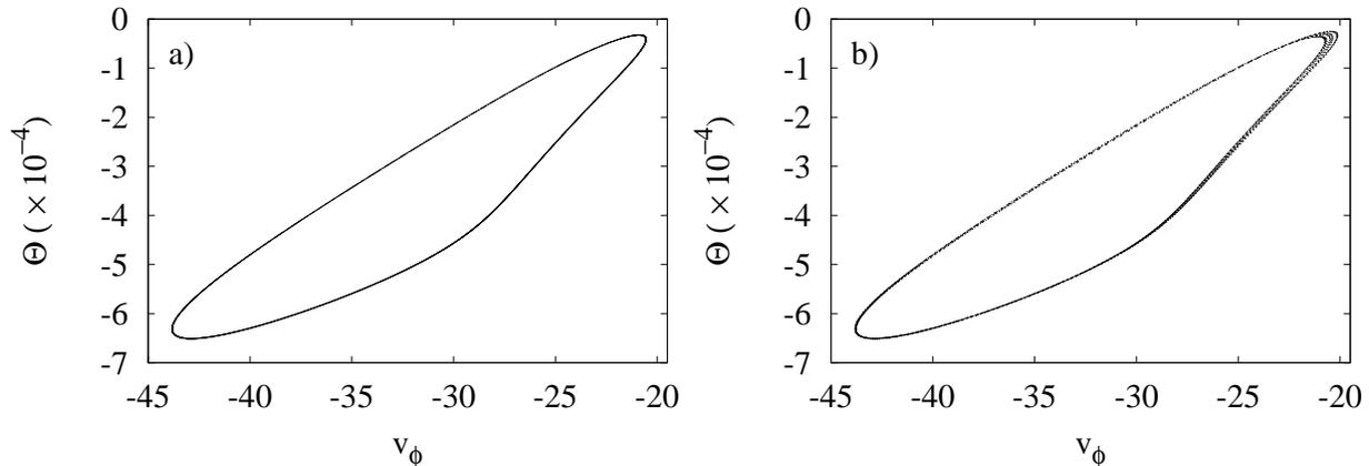
FIG. 5. Poincaré section at  $\Theta((r_o+r_i)/2, 0, 3\pi/8) = 0$  of the azimuthal component of the velocity field  $v_\varphi(r_i+(r_o-r_i)/7, 0, 3\pi/8)$  plotted versus  $\Theta$  at the same point. (a) Stable  $m = 1$  MRW at  $Ra = 2.15701 \times 10^5$ . (b) Stable three-tori bifurcated from the  $m = 1$  MRW at  $Ra = 2.15685 \times 10^5$ .
