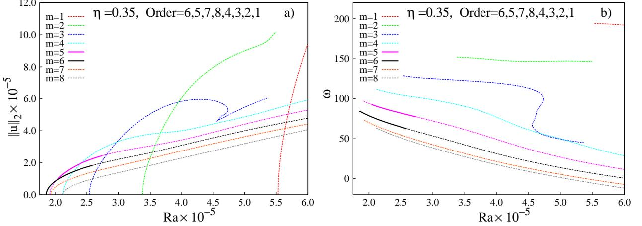
FIG. 1. Bifurcation diagram (taken from [31]) showing (a) the  $\mathcal{L}_2$ -norm of the RW and (b) the drifting frequency,  $\omega$ , both versus  $Ra$ .
