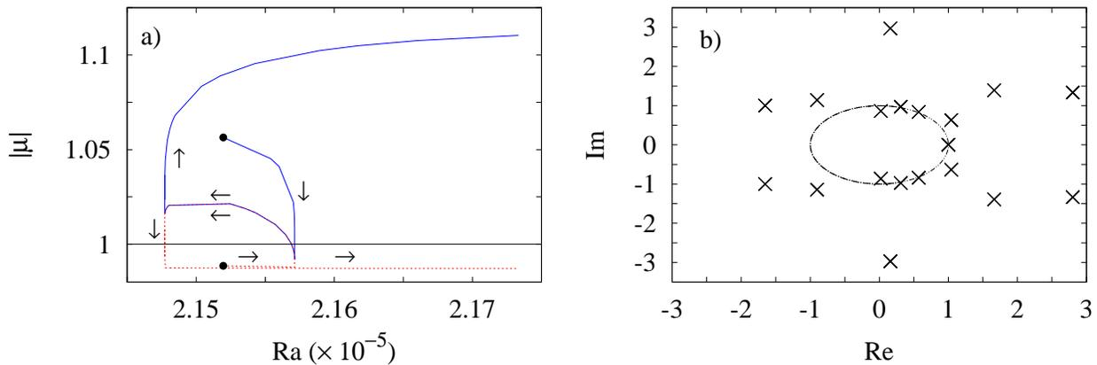
FIG. 4. (a) Modulus of the two leading Floquet multipliers versus  $Ra$ , for the solutions shown in the detail of Fig. 2(b). (b) Leading Floquet multipliers of the last solution calculated on the  $m = 1$  branch. The closed curve is the unit circle.
