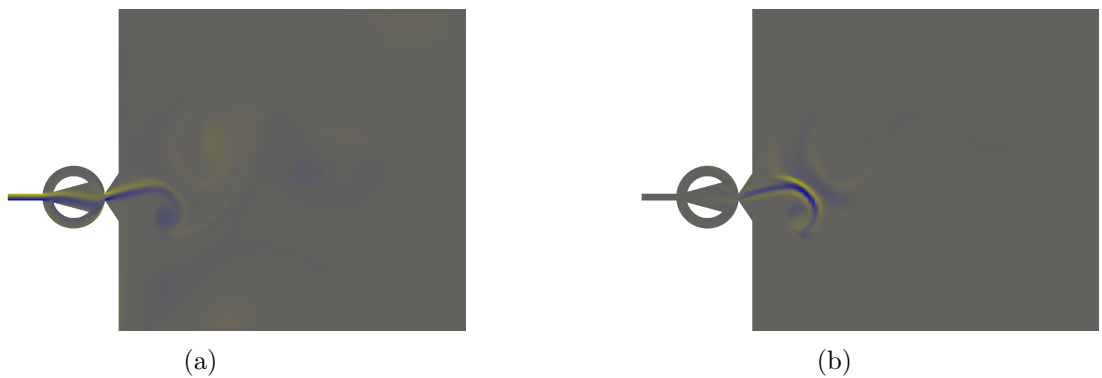
Figure 4.14: Vorticity field during the evolution of Fourier mode in the linear regime (a) instantaneous spanwise vorticity field of spanwise mean flow at Re=100 in the linear growth regime, \omega_z \in [-5, 5] ; (b) instantaneous crossflow vorticity field of Fourier mode at the same instant as that of mean flow at Re = 100 , \hat{w} \in [-1, 1]
